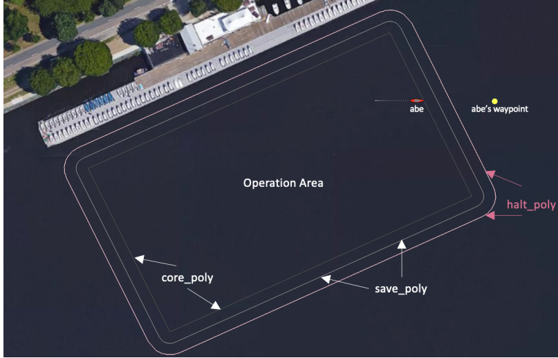
Figure 1: OpRegionV24 Behavior Regions: The operation area is defined by the core polygon. The buffer region is defined by the save polygon. The all-stop region is the area outside the halt polygon.
