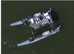
REx is an Unmanned Surface Vehicle (USV), made by Marine Advanced Robotics in California. REx is a Wave Adaptive Modular Vehicle (WAM-V). The MIT vehicle arrived in 2014 as part of the 2014 Robot-X competition in Singapore. It continues to be used for development of sensing and autonomy algorithms and software.
