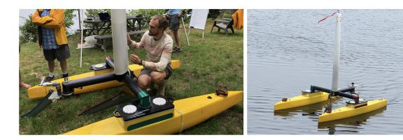
The Autonomous Sailboat is made by Marine Robotics, LLC, led by Walter Holemans in Maryland, supported by Joseph Curcio in Maine. An initial goal for building this boat is to provide a long-duration remote water sensing system to support the oyster aquaculture industry in Chesapeake Bay. The goal of the MIT team is to provide autonomy software to support this mission and autonomous sailing in general.
