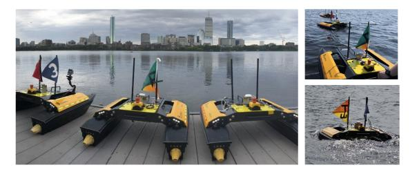
The Heron is a small unmanned surface vehicle (USV) made by Clearpath Robotics in Waterloo Canada. MIT has six Herons with plans for addition vehicles in the Spring of 2021. They are the primary teaching platform for MIT 2.680 taught each Spring Term since 2012.
