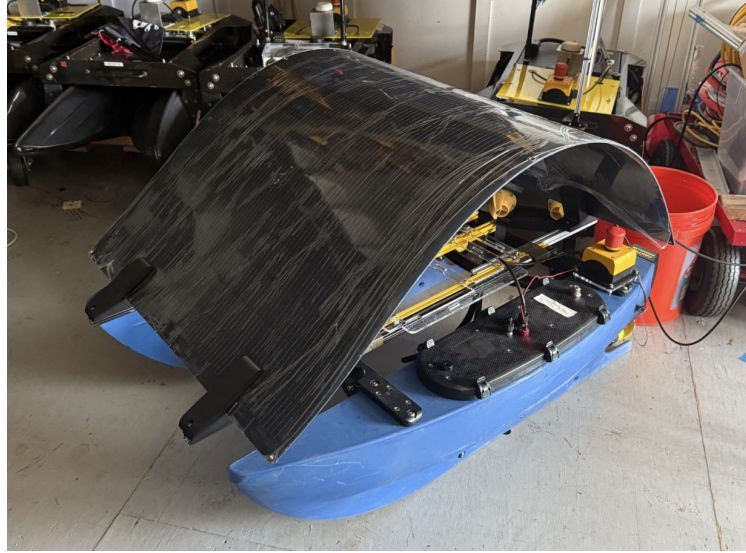
Figure 1: BlueBoat with 180W solar charging system.
