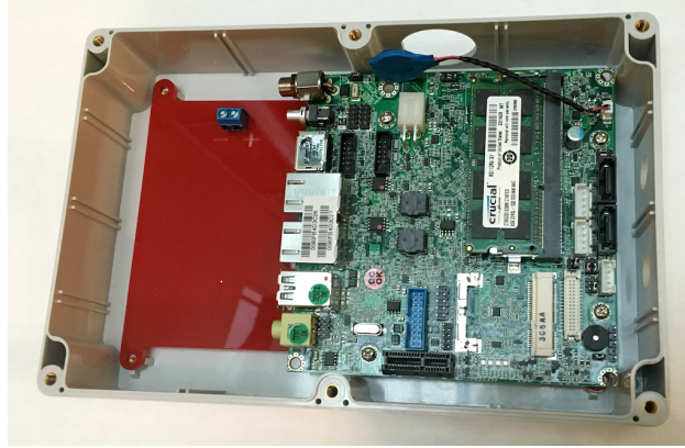
Figure 4: The Portwell Nano-6060 single-board computer fits tightly within the waterproof housing and is one possible computing option.
