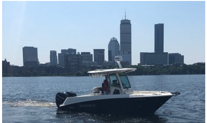
Figure 1. R/V Philos (RoboWhaler) is a mobile marine autonomy laboratory that is capable of collecting coordinated marine perception datasets. This marine vehicle operates in two modes manned and unmanned. While in the unmanned mode, the vessel becomes 'RoboWhaler' and is used for advanced autonomy and sensor fusion algorithm development
