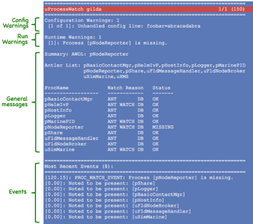
Figure 6: An appcast consists of four main parts: (1) configuration warnings, (2) run-time warnings, (3) general status report messages, and (4) run-time events. The bar at the top of the figure is rendered in red due to the presence of a run-time warning. The "1/1" on this line indicates one configuration warning and one run-time warning. The "(150)" on this line indicates that it is iteration #150 for this application. This image is a screen shot take from the uMACView utility described later.
