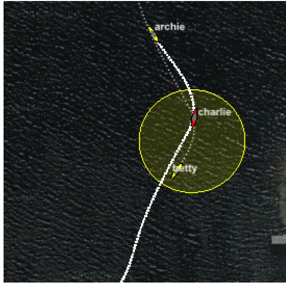
Figure 115: Using Range Pulse with uFldCollisionDetect: A range pulse is displayed in pMarineViewer with each detected collision.
