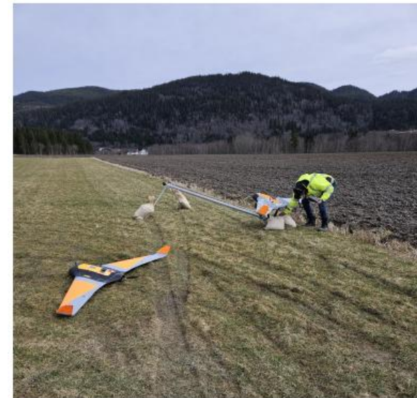
Rigging the two X8s
