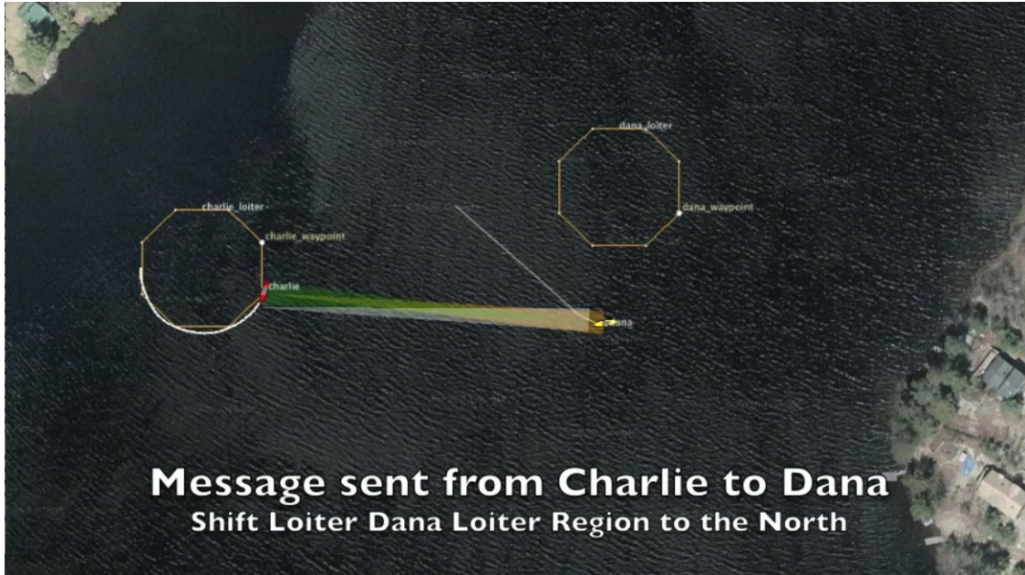
Figure 4: A simple two-vehicle baseline mission with both vehicles loitering at a fixed location, and inter-vehicle communications supported with uFldNodeComms running. A message is periodically sent from charlie to dana, indicated by the brief white comms cone between the two vehicles. When they are outside of comms range, no colored comms cones rendered, there are no inter-vehicle messages.
