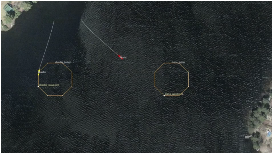
Figure 2: A simple two-vehicle baseline mission with both vehicles loitering at a fixed location. video:(0:18): https://vimeo.com/88522655
