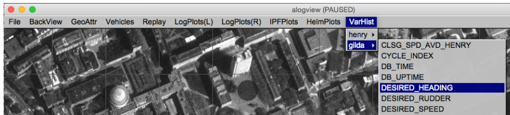
Figure 10: The VarPlot pull-down menu: is used for first selecting a vehicle and variable name, and launching the VarPlot window.
