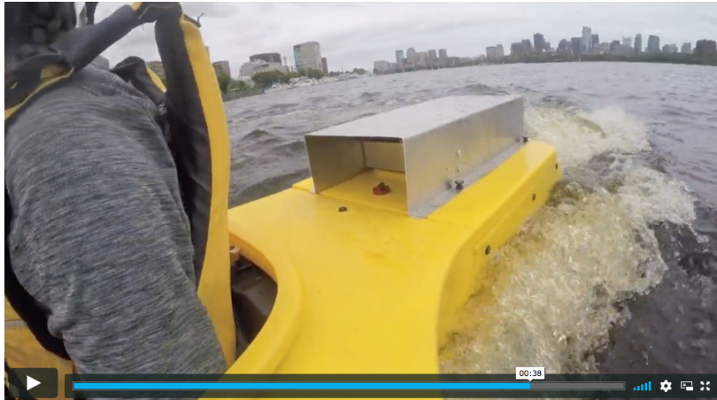
Figure 2: The MOKAI has been modified with covers over the air intake openings on the stern. video:(0:46): https://vimeo.com/222021219
