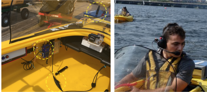
Figure 8: Each MOKAI is configured with a marine radio mounted in the boat as shown on the left. One line goes to the operator headset. The other line goes to an RF antenna mounted on the bow.
