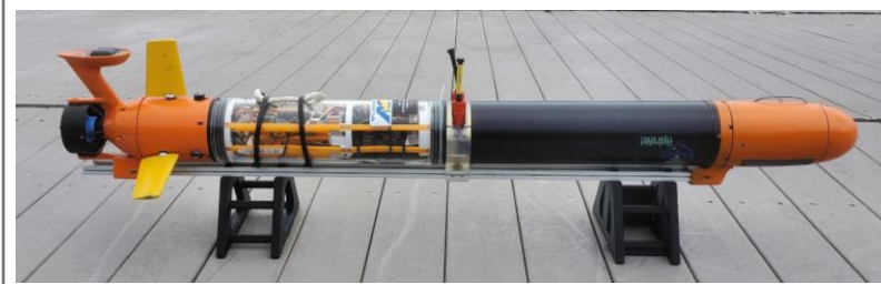
Base SeaBeaver + software defined acoustic modem payload
