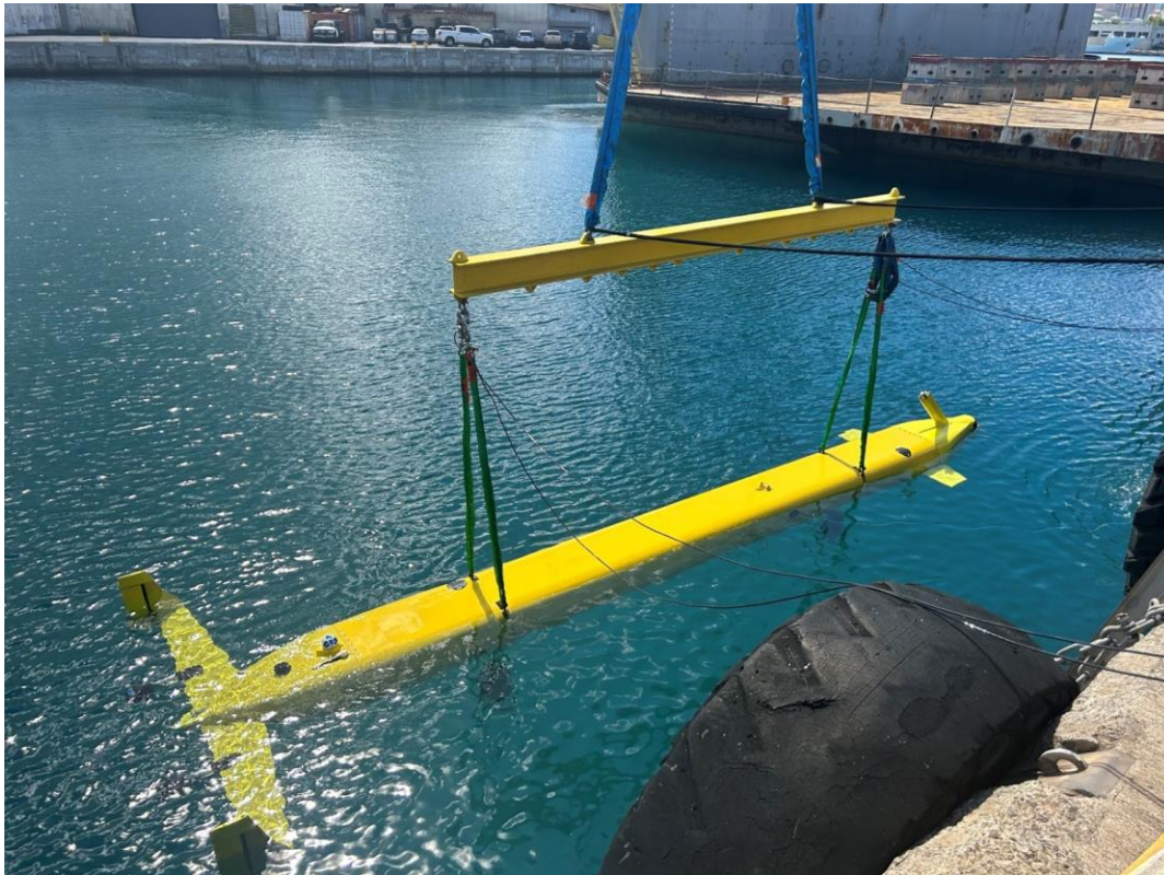
Scaled-down prototypes of DARPA Manta-Ray XL hybrid UUV
