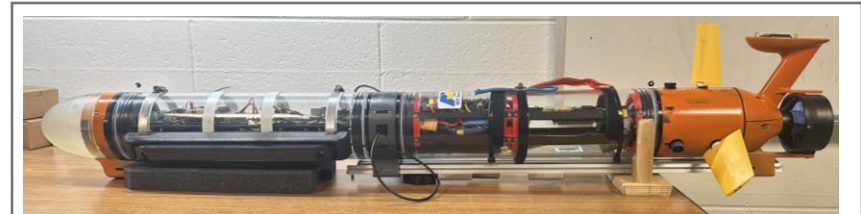
Base SeaBeaver + side scan sonar payload By University of Delaware
