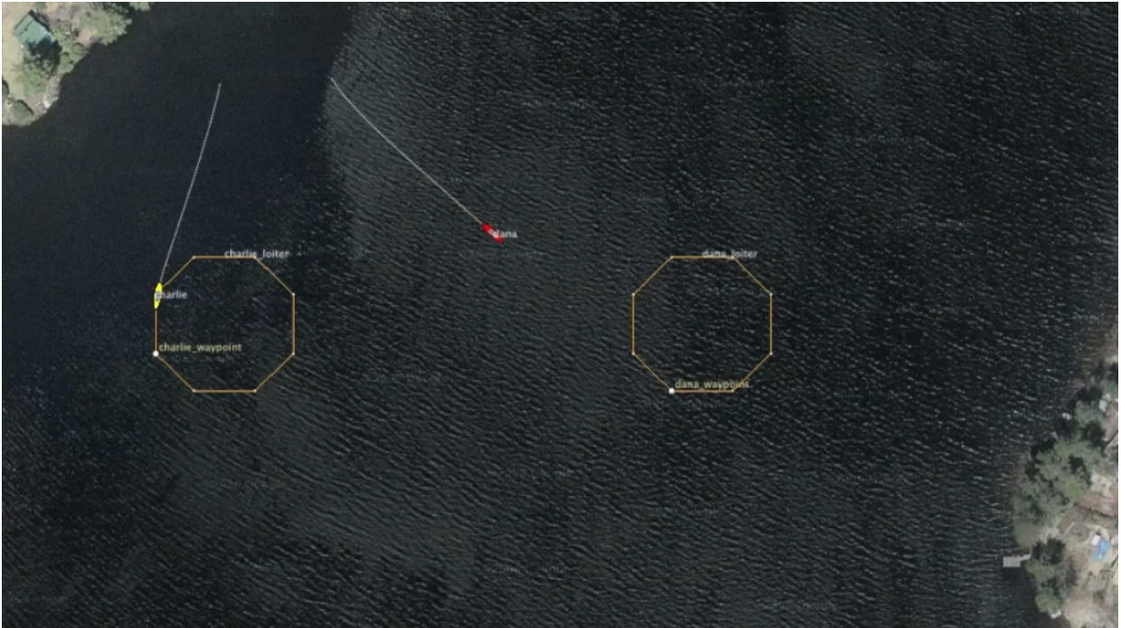
Figure 2: A simple two-vehicle baseline mission with both vehicles loitering at a fixed location. Video:(0:18): https://vimeo.com/88522655
