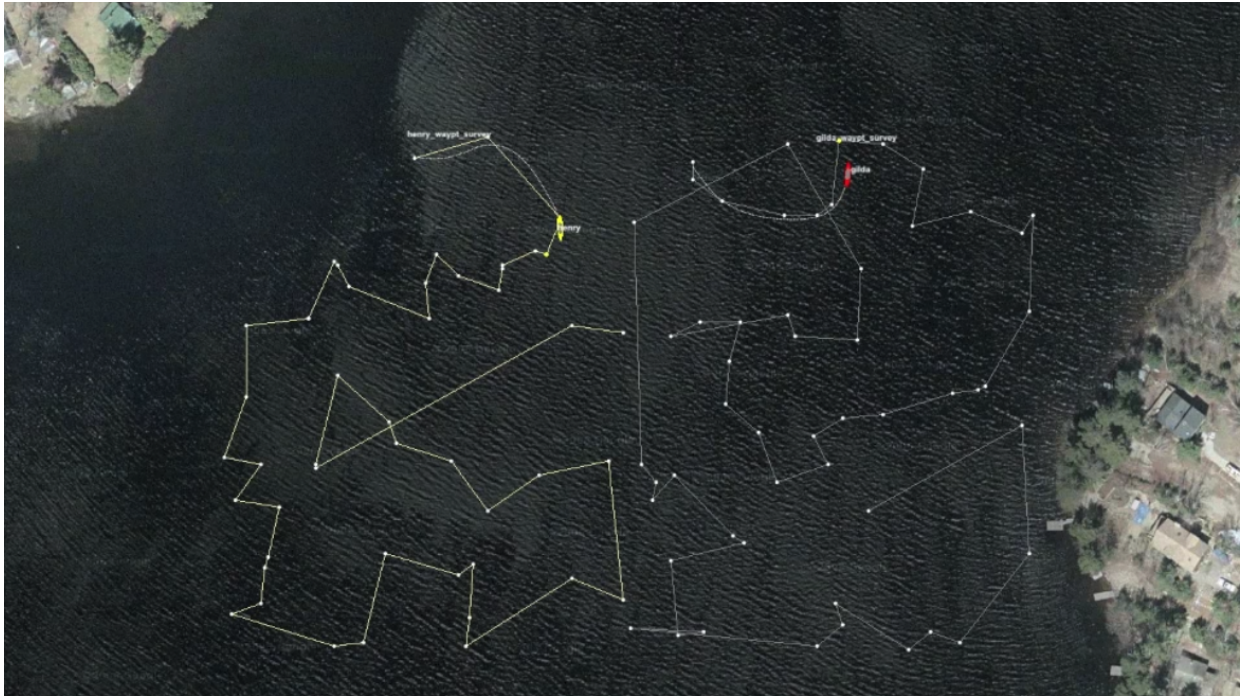
Figure 3: In the Distributed TSP Two mission two vehicles are assigned randomly chosen points in the region based on the section of the region. Therefore their paths do not overlap and the mission is somewhat more efficient.
