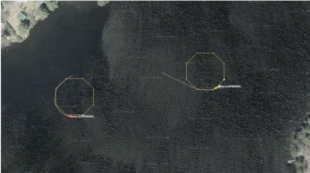
Figure 4: A simple two-vehicle mission connecting two loitering vehicle communities, and a shoreside community, using the uField Toolbox utilities for coordinating the pShare connections.
