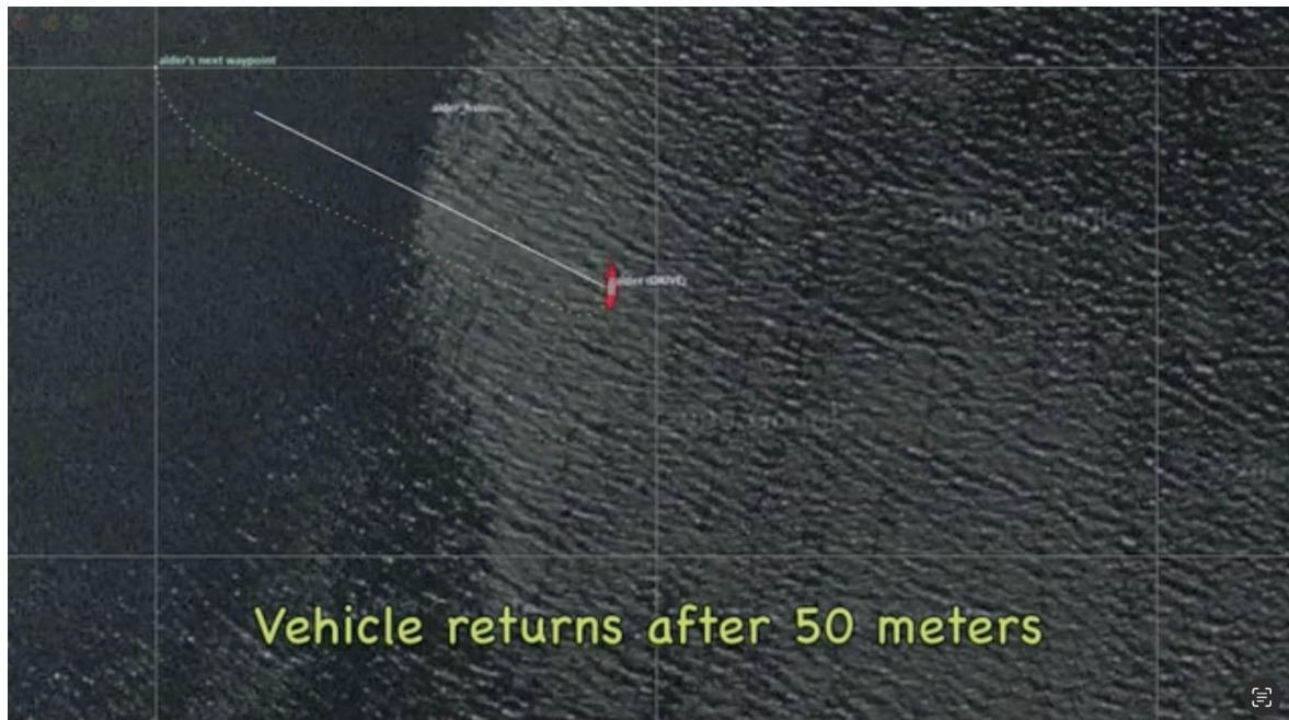
Figure 4: The Alder mission with odometry. The vehicle begins to travel to point (100,-50), but returns home early based on odometry distance.
