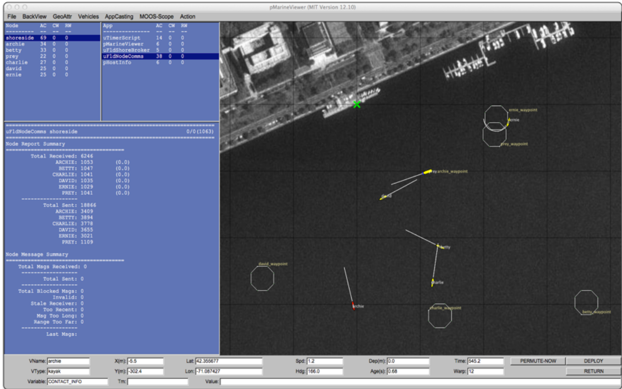
Figure 60: The pMarineViewer utility has an appcasting viewing capability very similar to uMACView embedded in the viewer. The rendering of the appcasting panes may be toggled on/off with the 'a' key.
