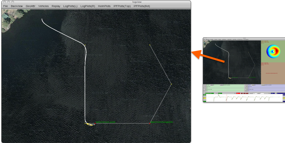
Figure 79: The OpArea panel of the alogview tool: Vehicle position(s) for a given point in time are rendered along with vehicle trajectory history and certain geometric visual artifacts such as points, polygons and line segments that may have been posted by the helm or another MOOS process. The image in this figure can be replicated exactly by launching alogview on the alpha.log file from the Alpha mission distributed with the MOOS-IvP source code, launched with the --nowtime=144 command line option.
