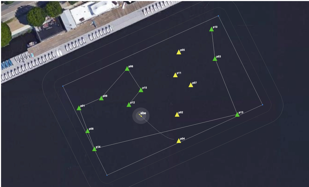
Figure 3: The swimmer locations shown are from swimmer file mit_02.txt . The vehicle proceeds to each point, in a greedy path tour, and then returns home.
