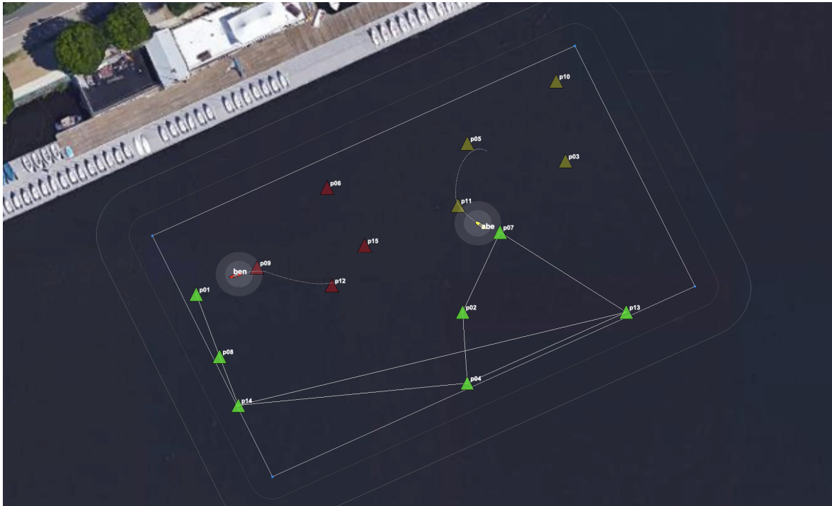
Figure 4: Two vehicles are given the same set of swimmers and locations. They each depart at the same time, each using a greedy path to traverse the set of swimmer locations and tally rescues. This mission was run at 10x realtime.
