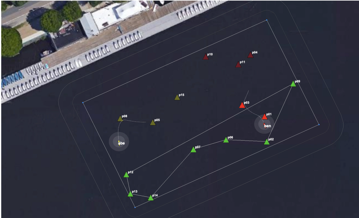
Figure 4: Two vehicles are given the same set of swimmers and locations. They each depart at the same time, each using a greedy path to traverse the set of swimmer locations and tally rescues. Swimmers rescued by the yellow vehicle are indicated by the light-yellow markers. Swimmers rescued by the red vehicle are indicated by light red markers. If some markers are brighter in color this indicates a differential between total swimmers rescued between the two vehicles. This mission was run at 10x realtime.
