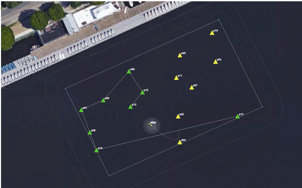
Figure 2: The vehicle proceeds to each point, in a greedy path tour, and then returns home.
