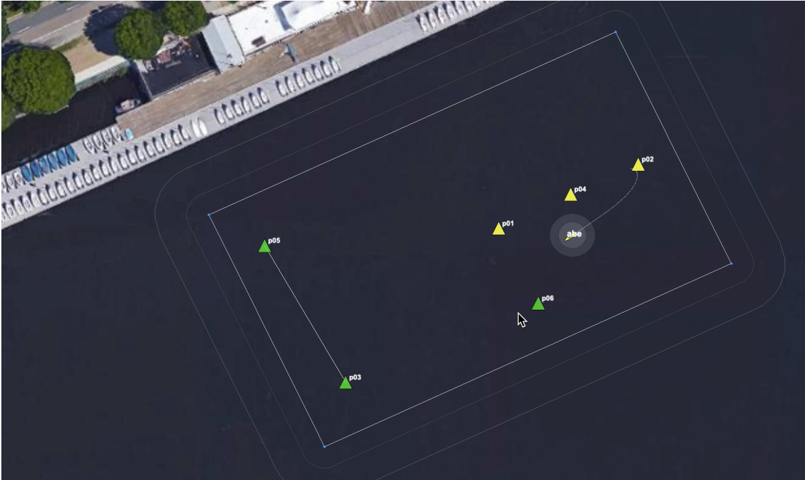
Figure 3: The swimmer locations shown are from swimmer file mit_03.txt . The vehicle proceeds to each point, in a greedy path tour. During the mission, a new point is added by the shoreside user, and the path is adjusted. Finally the vehicle then returns home.
