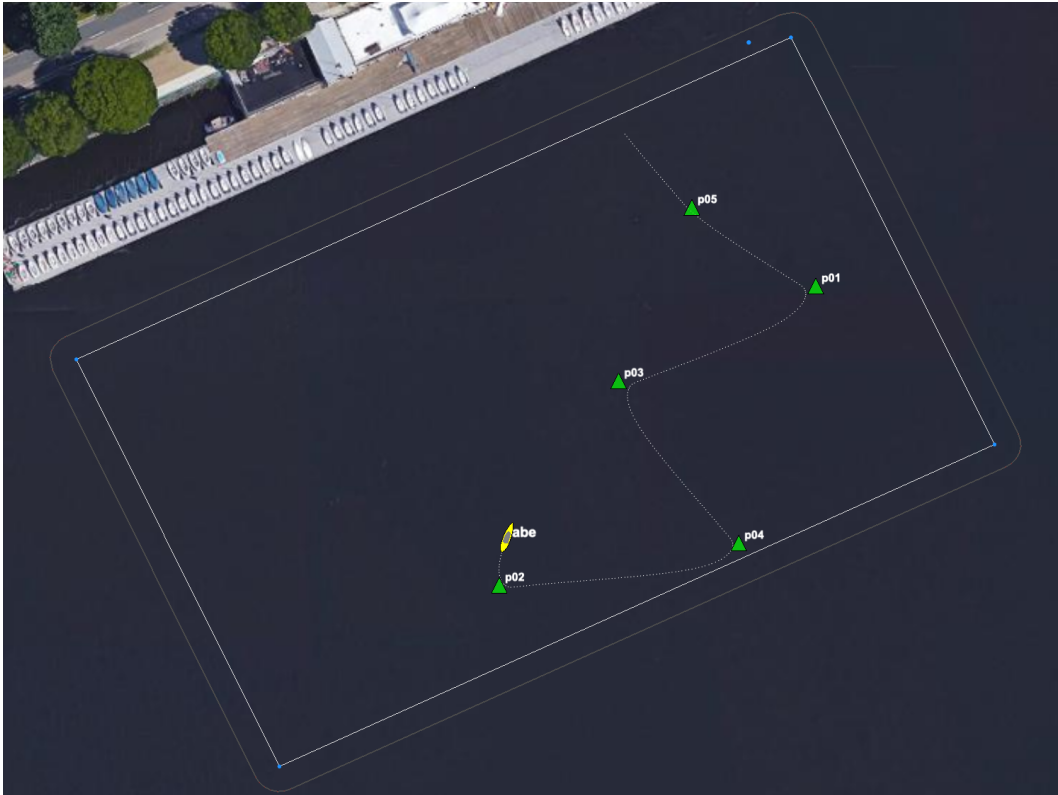
Figure 6: In the first baseline mission, the vehicle will proceed to visit all five swimmer locations, before returning home. The circle moving with the vehicle represents the sensor range for performing rescues.
