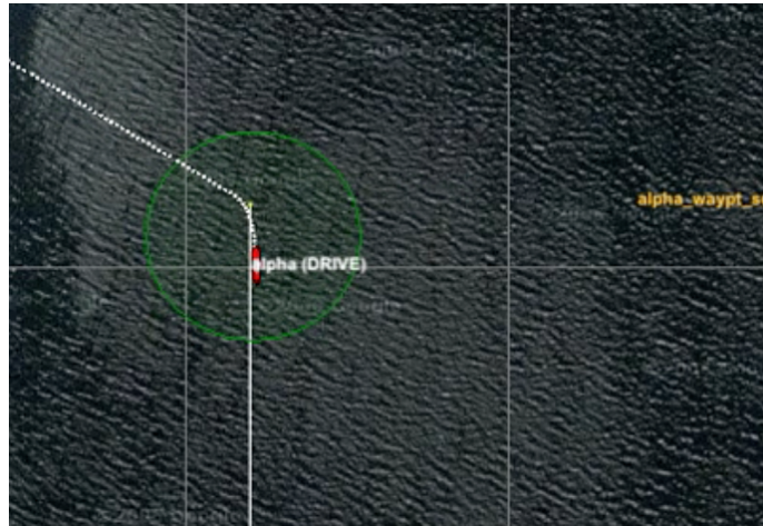
Figure 1: The Pulse Behavior: The behavior simply generates a range pulse after it observes that a waypoint has been achieved. The range pulse is a posting to the variable RANGE_PULSE .
