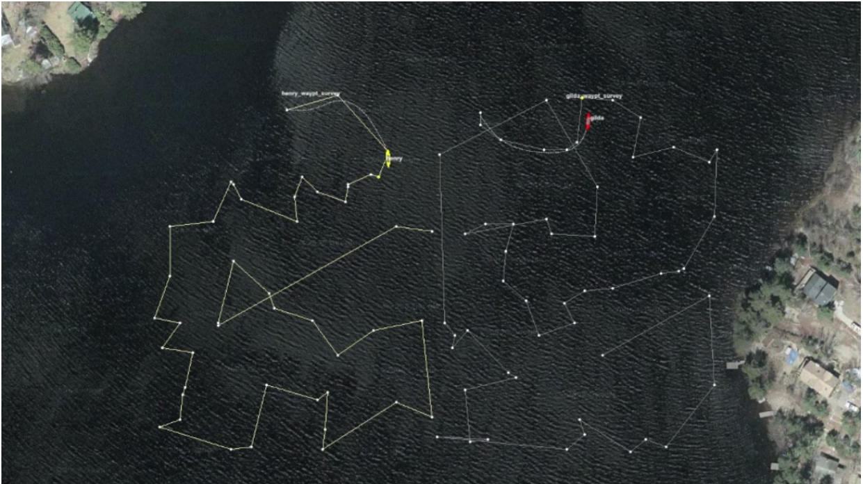
Figure 5: In the Distributed TSP Two mission two vehicles are assigned randomly chosen points in the region based on the section of the region. Therefore their paths do not overlap and the mission is somewhat more efficient.
