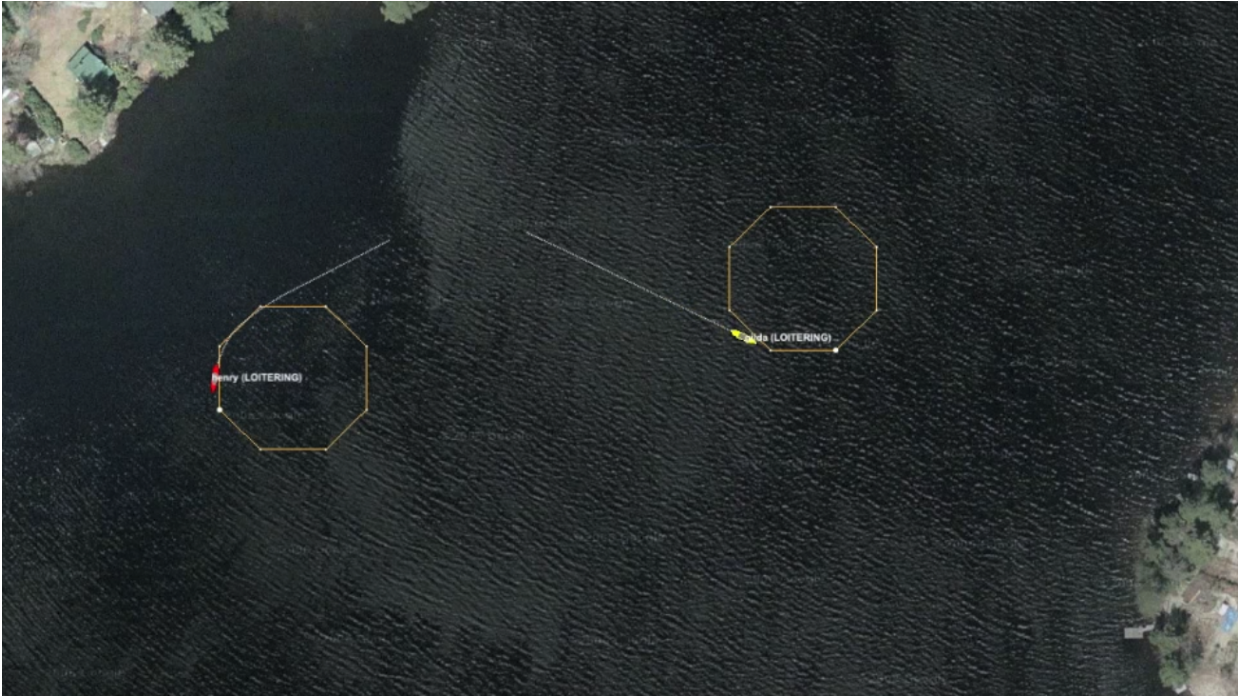
Figure 6: The Henry Gilda Refuel mission has two loitering vehicles. When the user commands the vehicles to return, they return to their starting point and station keep for 60 seconds and automatically re-deploy afterwards. As with the baseline mission, both vehicles have their own MOOS community, connected to a shoreside community, with the connections coordinated using the uField Toolbox utilities.
