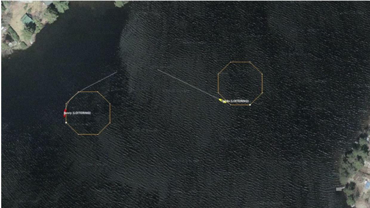
Figure 5: The Henry Gilda Refuel mission has two loitering vehicles. When the user commands the vehicles to return, they return to their starting point and station keep for 60 seconds and automatically re-deploy afterwards. As with the baseline mission, both vehicles have their own MOOS community, connected to a shoreside community, with the connections coordinated using the uField Toolbox utilities.
