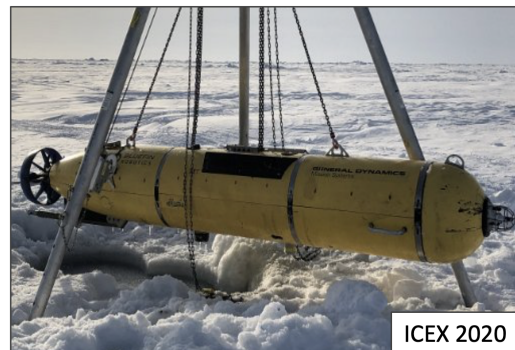
Figure 6: The Bluefin 21-inch UUV have in recent years been primarily used for participation the Navy's ICEX experiments in the Arctic.
