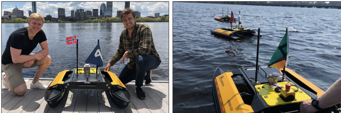
Figure 5: The Clearpath Robotics Heron M300 USV, similar to the M200, used custom-made pontoons and hull frame. The M300 computer section is removable however, and can be seamlessly swapped between vehicle bodies. Clearpath supported an "MIT variant" which included an E-stop button. MIT also created its own payload cover with mounts for the GPS receiver and IMU. (On the left, Simen Overeng, Oliver Os, Norwegian visiting students, Spring 2019.)
