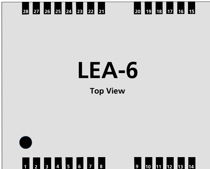
Figure 2 LEA-6 Pin Assignment
