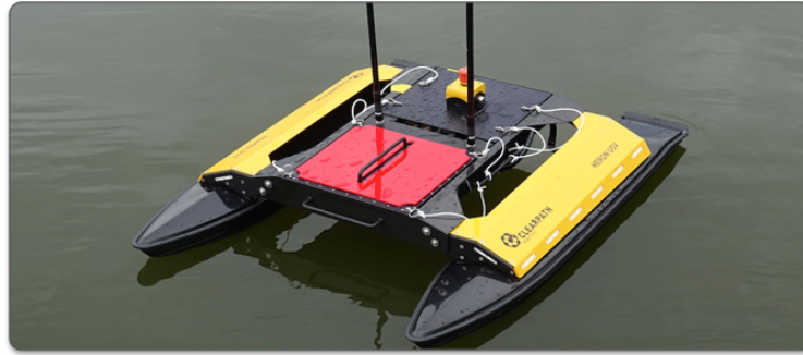
Figure 4: The Heron M300: The Heron M300 unmanned surface vehicle serves as the robotic teammate.
