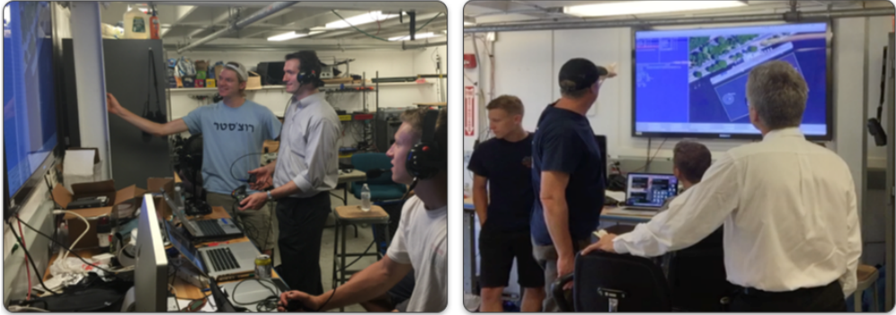
Figure 7: Aquaticus Multi-User Simulation: Users are connected to the simulation with same headsets worn on the water. A simulated vehicle is under joystick control with functionality similar to the joystick control of the thrusters on the actual vehicle.
